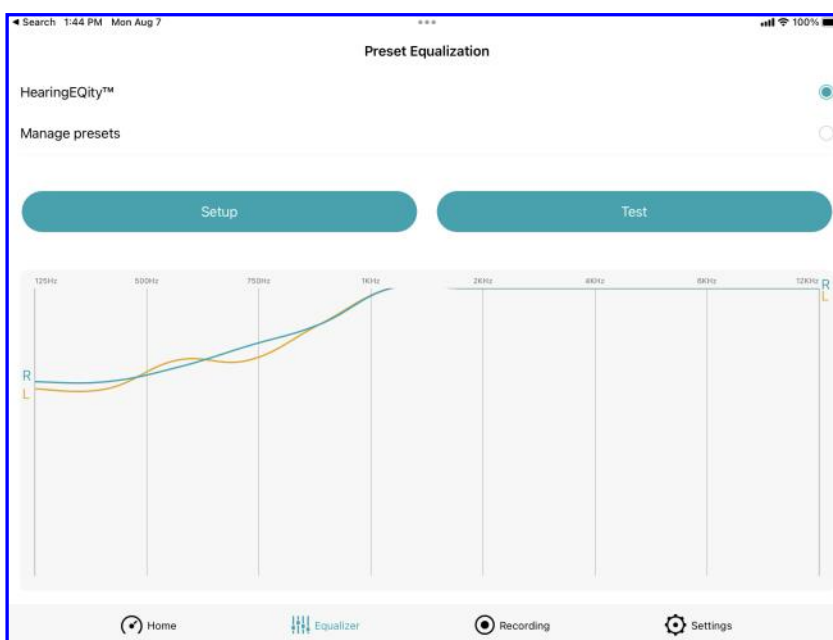
The iPad app shows a graph with the dialed-in frequency compensation. For me, it was maxed out at 1kHz.
